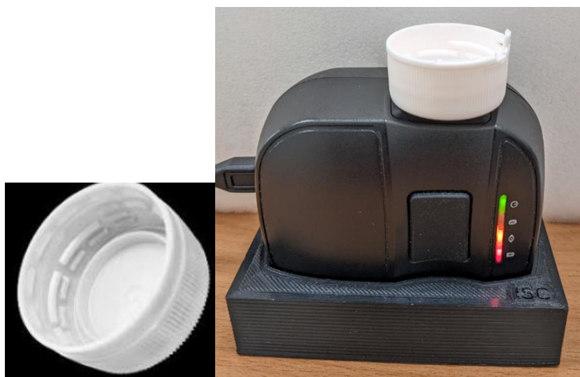
Figure 3.2 Diffuse Reflective Measurement of Plastic Bottle Cap (HDPE)
