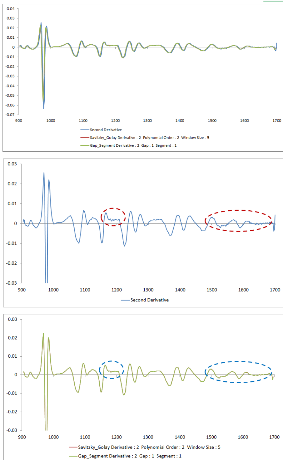
Figure 4.8 Savitzky-Golay and Gap-Segment Avoid Noise Enhancement
