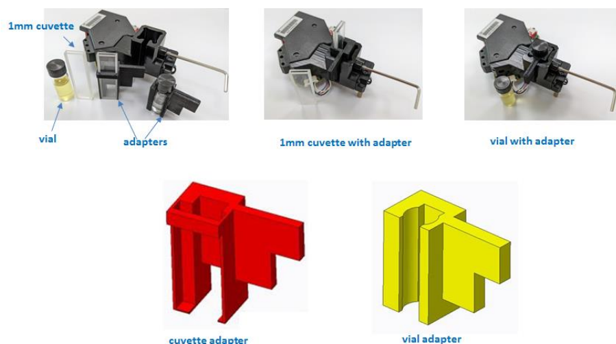
Figure 3.9 Alignment of Sample Vial and Short Path Length Cuvette
