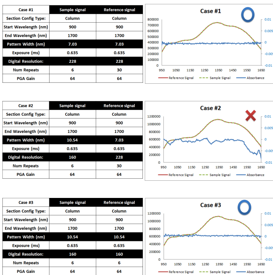
Figure 2.11 Cases with Matched or Unmatched Scan Configuration
