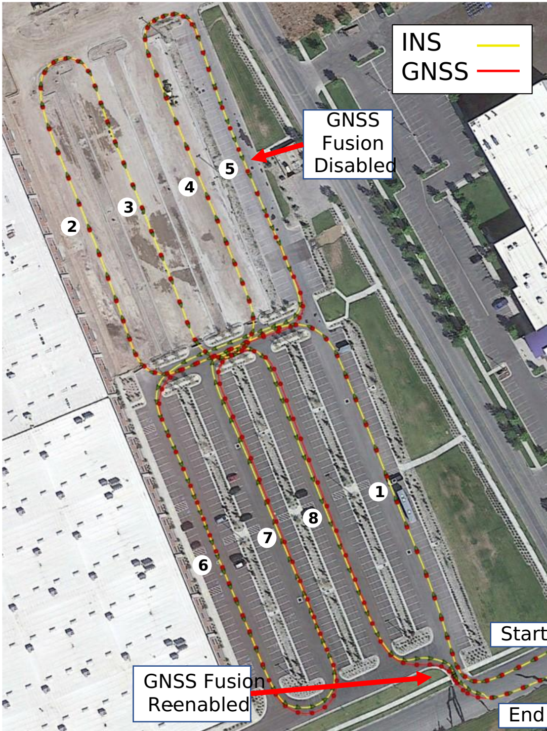
In the drive the car starts and ends the drive at the bottom right corner of the image. The numbered path segments show the order of travel. GPS fusion was disabled in the middle of path segment 5.
